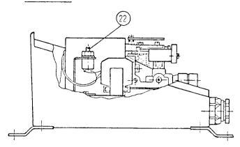
After the zero is adjusted, increase the input to 10 V=100 % and adjust the output to 4 bar = 100 % with
