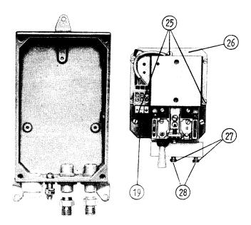
Remove the electrical leads at the terminals (19).
