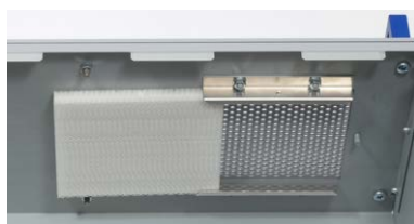
Figure 14: Air filter, already moved, and ventilation holes of the C-887
