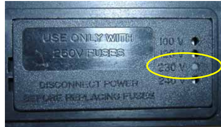
Fig. 4: Factory-set voltage selection, here: 230V
