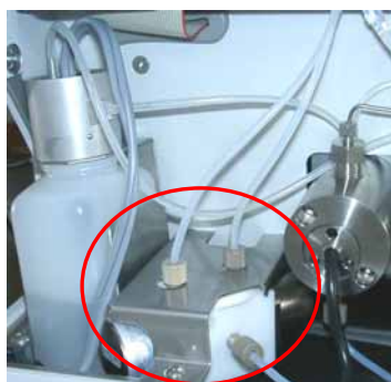
Left pump block
