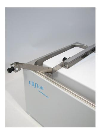
$\label{eq:conjunction} \mbox{Fit $``Z''$ shaped bracket to Float Assembly, this in conjunction with a motion sensor and data logger can record pulmonary ventilation.}$
