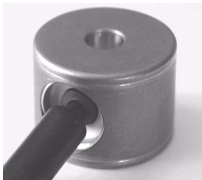
Figure 43. Removing the used primary piston seal
