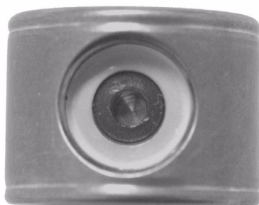
Figure 48. View showing the piston bore with a properly seated seal
