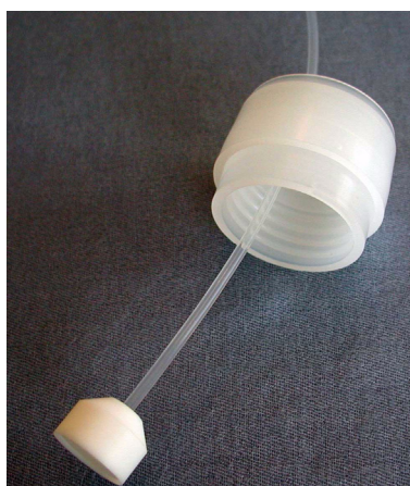
Figure 13. Solvent reservoir cap assembly
