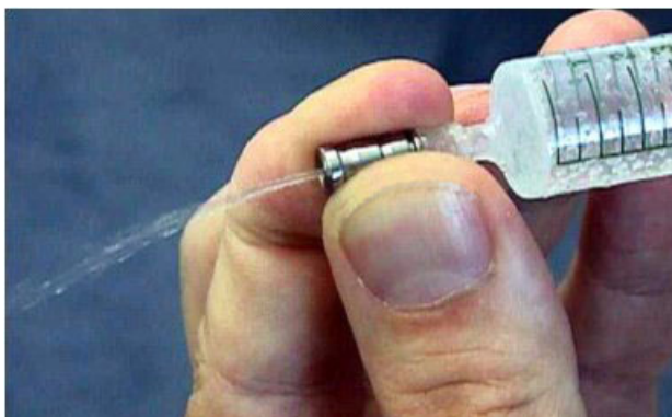
Figure 41. Cleaning the check valve
