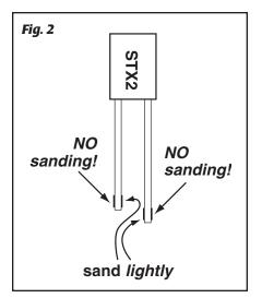
**3.** Lightly rub the voltage electrode (silver pellet on the inner surface near the electrode tips) of the **STX2** with the 600-grade Ultra Fine sandpaper provided (see Fig. 2). Only a very thin surface layer of the pellet should be removed. Repeated rubbing will eventually remove the Ag/AgCl pellets. When rubbing no longer improves the voltage readings, the electrode should be replaced. In the absence of 600-grade sandpaper, an ink eraser may be substituted to clean the electrodes.
