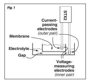
it touches the bottom of the dish each time, the reproducibility of the measurements is significantly improved. Even small differences in the apparent fluid resistance may occur if the depth to which the electrode tips are immersed varies.
