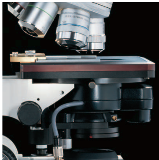
The newly designed industry stage with a travel range of 76 x 50 mm. 4" x 4", 6" x 4" and 6" x 6" stages are available for special applications. There is also a special stage for extra tall samples up to a height of 90 mm.
