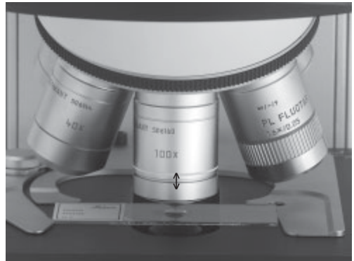
Fig. 44 Immersion objective (locked)
