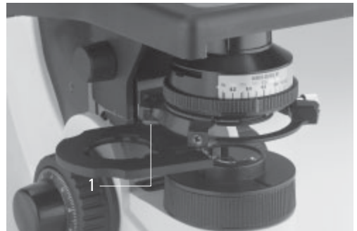
Fig. 19 Assembly of polarizer holder
