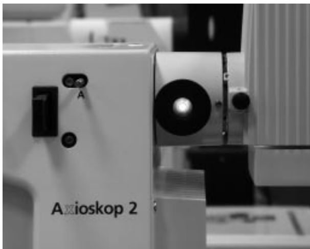
Fig. 2-20 Focal spot imaging via adjusting aid and knurled knob for focusing
